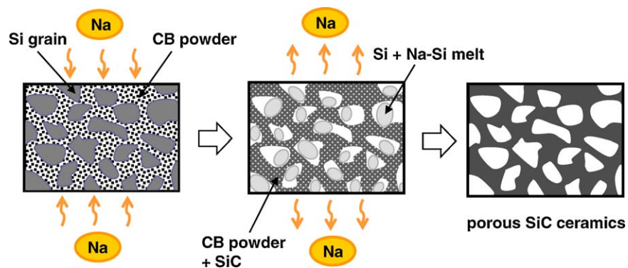
Fig. 5. Schematic illustration of the porous SiC ceramics formation process using Na vapor and Si grain templates.
